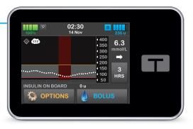
When the Sleep Activity is enabled, the algorithm narrows and lowers the range of treatment values to 6.25-6.7 mmol/L when determining whether to decrease, stop, or increase basal insulin delivery.
